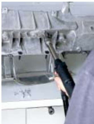
Assembly into cast magnesium beam
