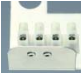
PVC connector block in air conditioning unit
