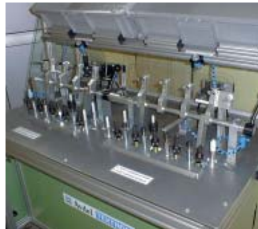
10 placing heads to assemble automotive sealing strips
