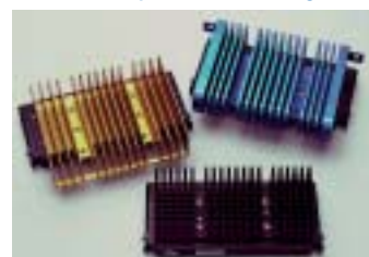
Heatsinks to processor cartridges
