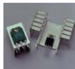
Semi-conductors to heatsinks and printed circuit boards
