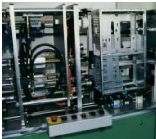
29 placing heads to assemble computer chassis
