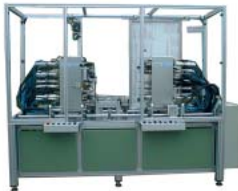
23 placing heads to assemble a computer chassis
